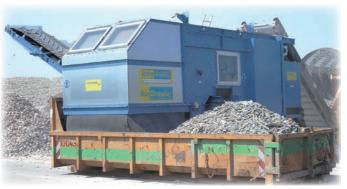
sorting Ferrous and non-ferrous metals have experienced a rapid development in value. It is almost always worth sorting. Over-belt magnets, the magnetic drum and the container-mobile non-ferrous materials separating equipment pay for themselves in a short amount of time.
