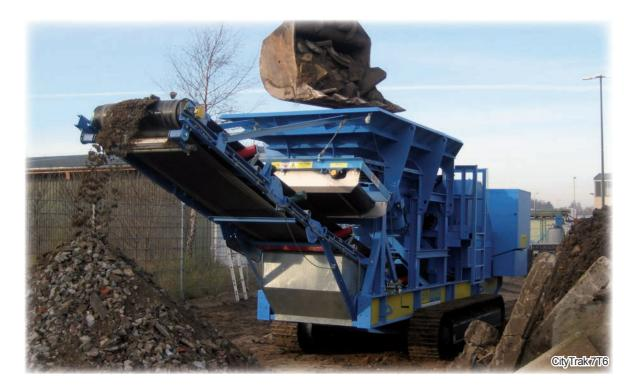
Well established, both nationally and internationally, in compact recycling and natural rock; the CityTrak 7T6 offers the best conditions for reducing coarse material to the desired grain size with low wear.
